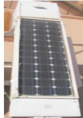
Fig.7. Photograph of the Prototype of covered PVT collector at URAER Unity, Ghardaia
