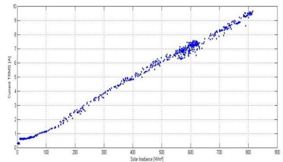
Fig. 5(b) Current TRMS measurement Vs solar irradiance
