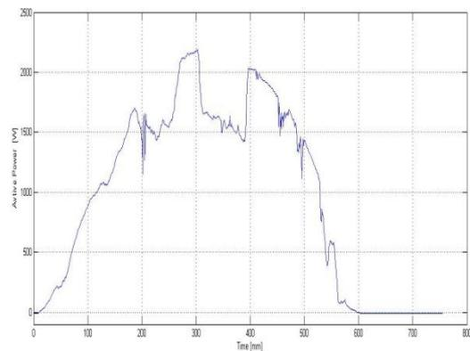
Fig. 3(b) Active Power measured for a day with an average solar irradiance
