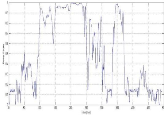
Fig. 4(d) Power Factor measured for a day with a low solar irradiance
