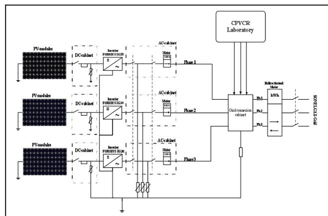
Fig. 1. Diagram of the grid-connected PV-system of CDER.
