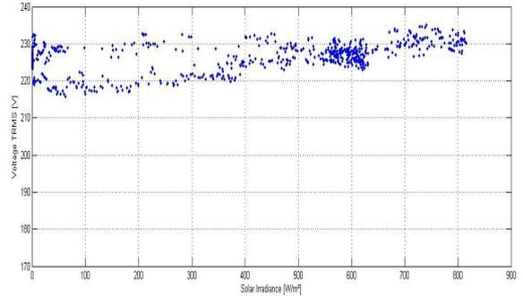
Fig. 5(a) Voltage TRMS measurement Vs solar irradiance
