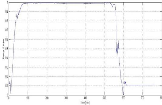
Fig. 3(c) Power Factor measured for a day with an average solar irradiance
