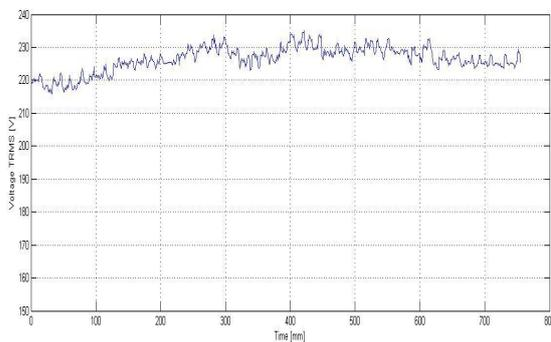
Fig. 3(e) Voltage TRMS measured for a day with an average solar irradiance
