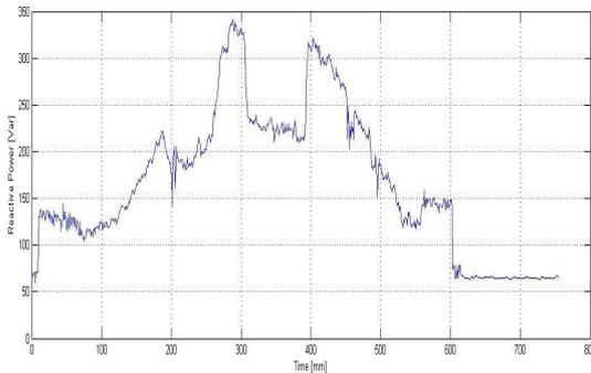
Fig. 3(d) Reactive Power measured for a day with an average solar irradiance
