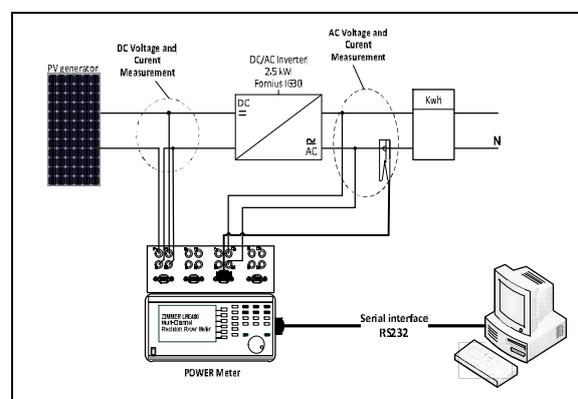
Fig. 2 Overview of the PV sub-array and the devices constituting the monitoring system
