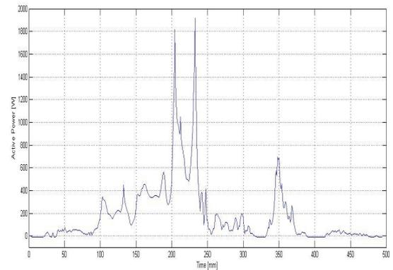
Fig. 4(b) Active Power measured for a day with a low solar irradiance
