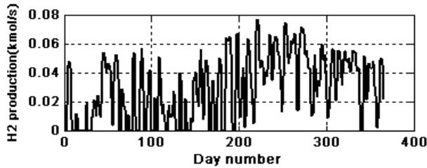
Fig.12: hydrogen production.
