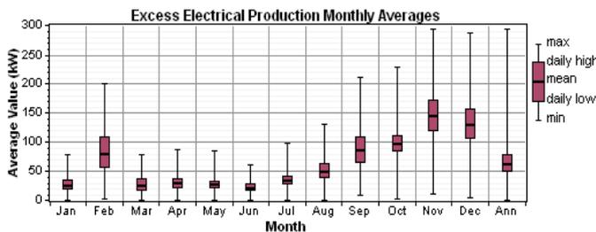
Fig.19: Excess electrical production monthly average
