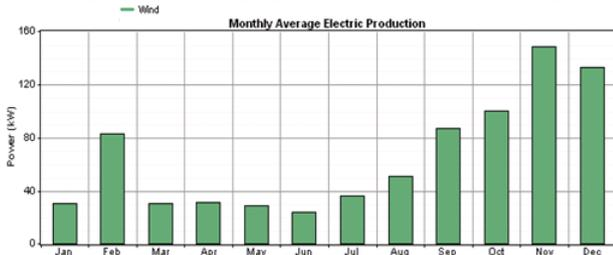
Fig.18: Monthly wind generator energy production.
