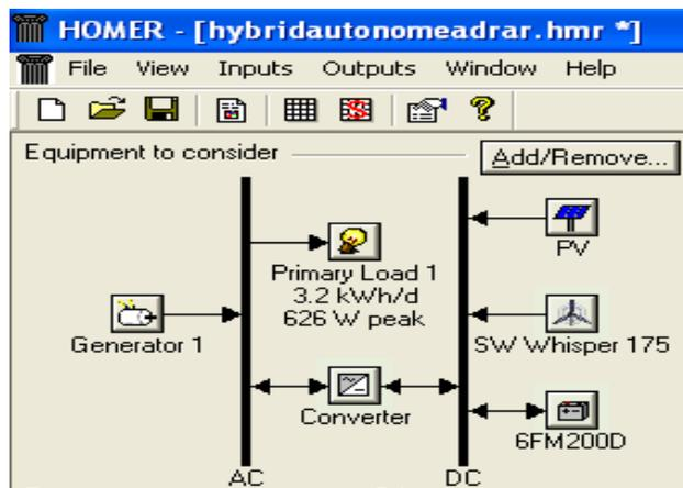
Fig. 1: Proposed hybrid system in HOMER
