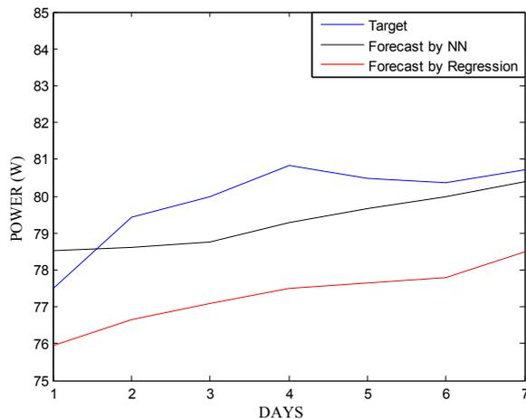
Figure 6. PV Power Forecasting Using Model 2
