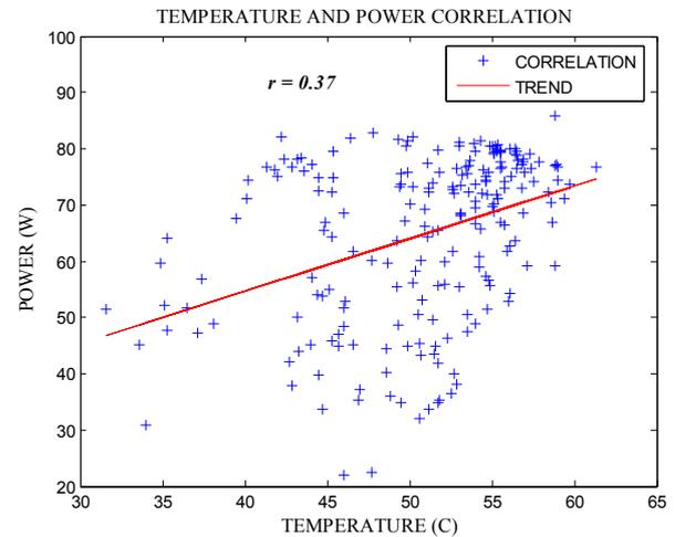
Fig. 3 Temperature vs. Power correlation
