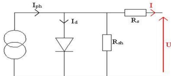
Fig. 1 : Equivalent circuit of a photovoltaic cell
