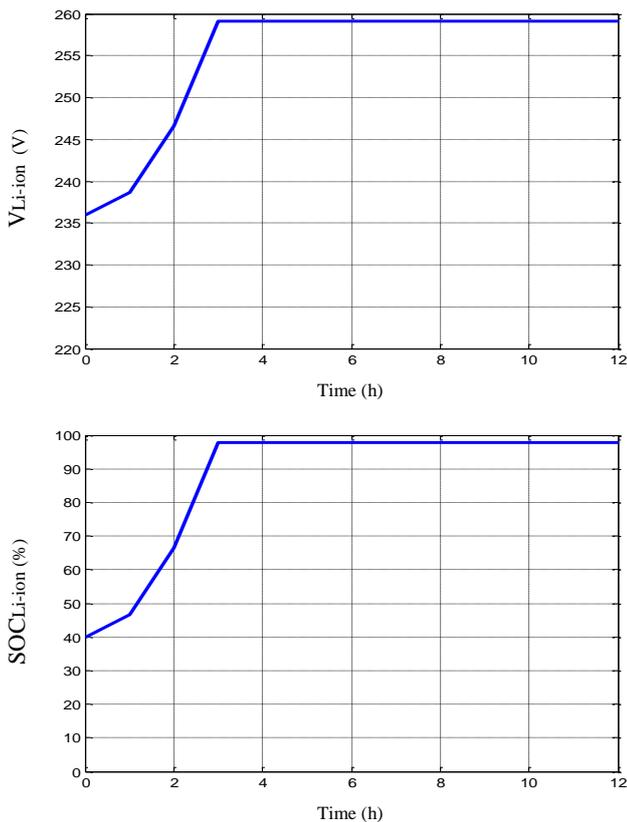
Fig. 11 : Batteries pack voltage and state of charge
