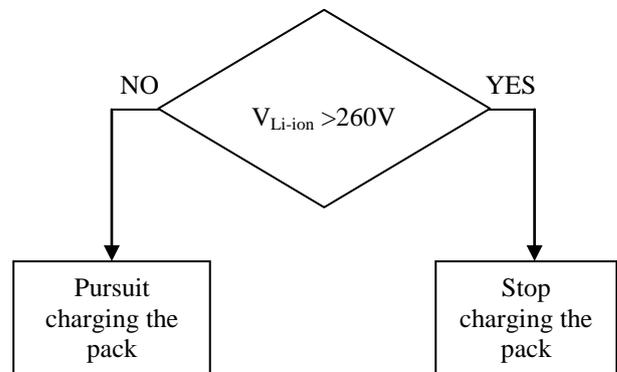
Fig. 4 : Principle of the supervision system
