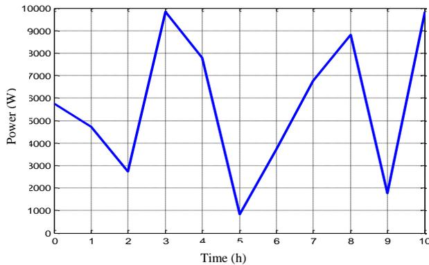
Fig. 7 : Maximum power that can be provided by the photovoltaic source
