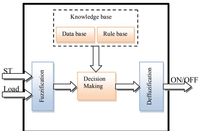
Fig.4. Fuzzy Logic Controller Design
