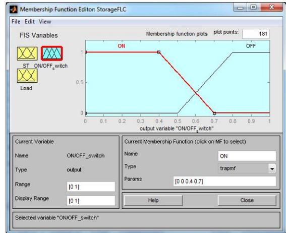
Fig.9. Membership function for the ON/OFF switch of the pump
