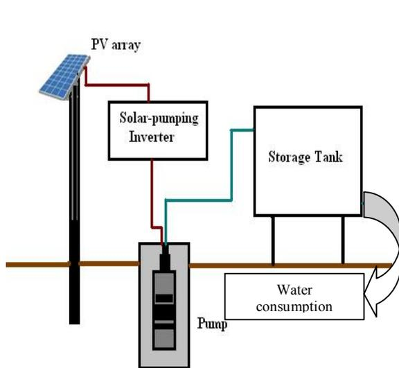
Fig.1. Global PV water pumping system configuration
