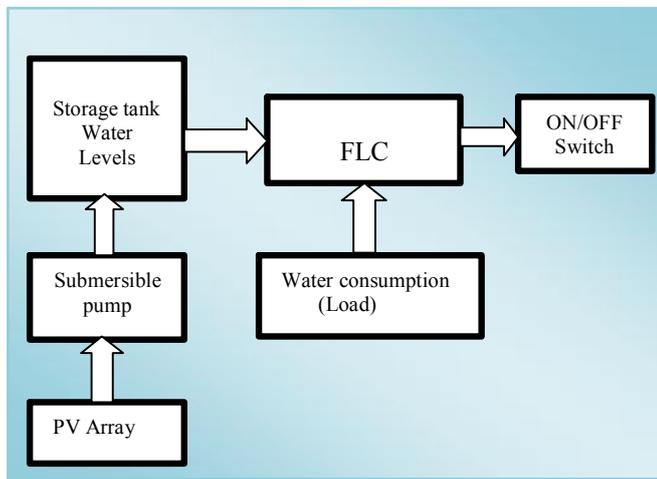
Fig.3. Synoptic of the control water management
