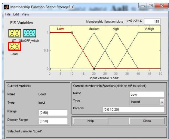
Fig.8. Membership function for the load (Load)
