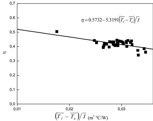
Fig. 3 Characteristic graph of the Maximum useful efficiency of the system
