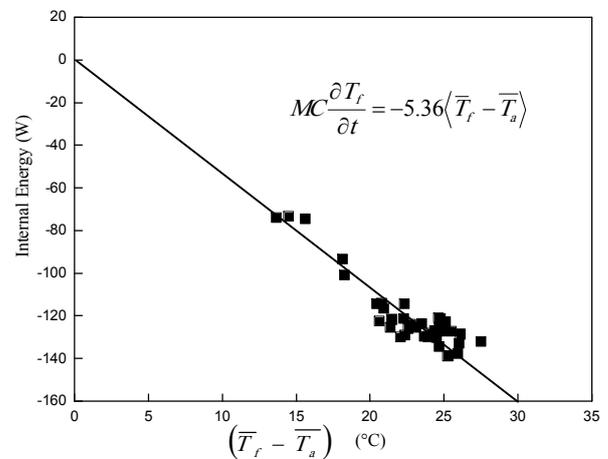
Fig. 4 Variation of the internal energy at night as function of  $(\bar{T}_f - \bar{T}_a)$
