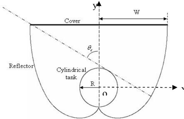
Fig. 1 Cross section of ICS system
