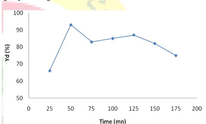
Fig. 2 Yields of sunflower oil transesterification according to reaction time
