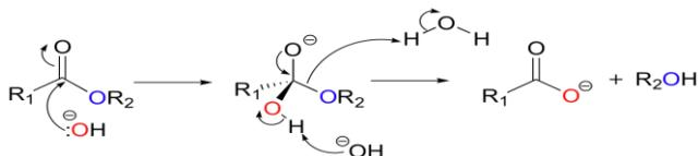
Fig. 3 Hydrolysis reaction of esters in due to the water formed during the dissolution of sodium hydroxide in methanol
