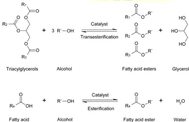
Fig. 1 Transesterification and esterification reactions carried out during biodiesel production from triacylglycerols or free fatty acids
