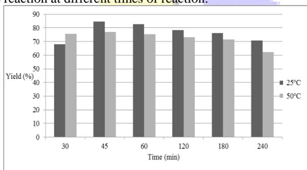
Fig. 2 Effect of reaction temperature on the yield of FAEE.
