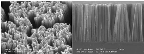
Fig1. Plan (a) and cross section (b) SEM image of p-SiNWs
