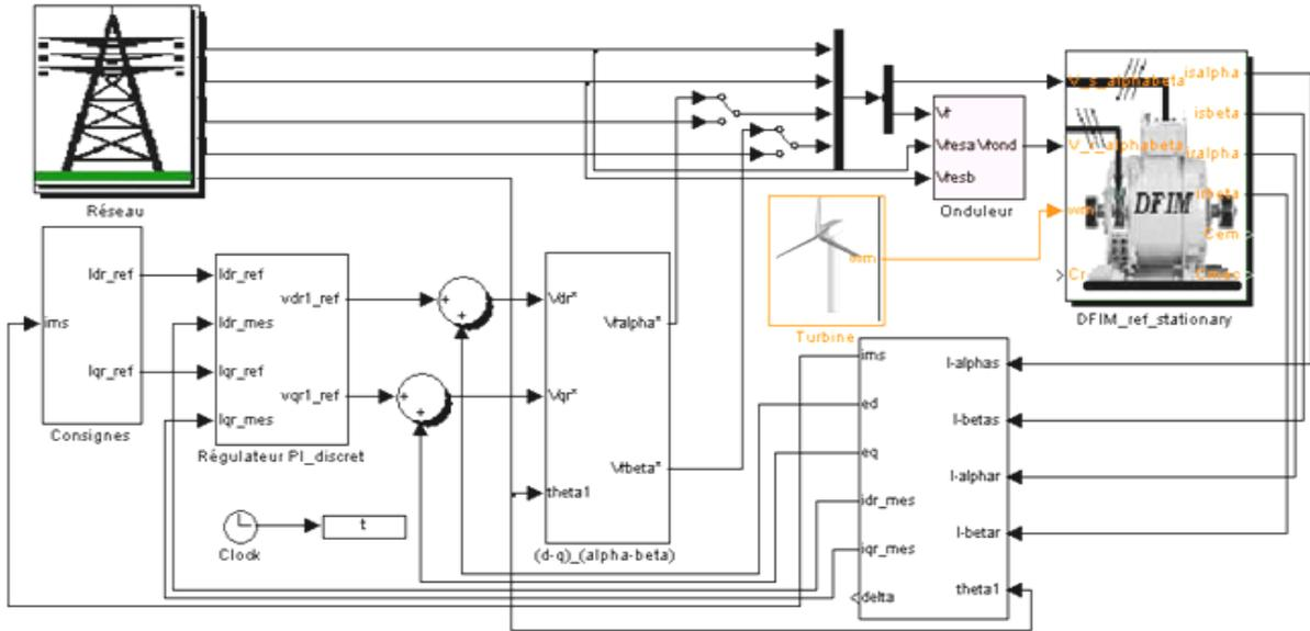
Fig.2 Simulation Scheme within Matlab/SIMULINK Environment.
