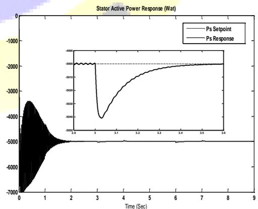
Fig.5. Stator Active Power Response
