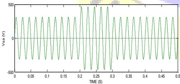
Fig10. Source voltages with 50% voltage swell in phase A
