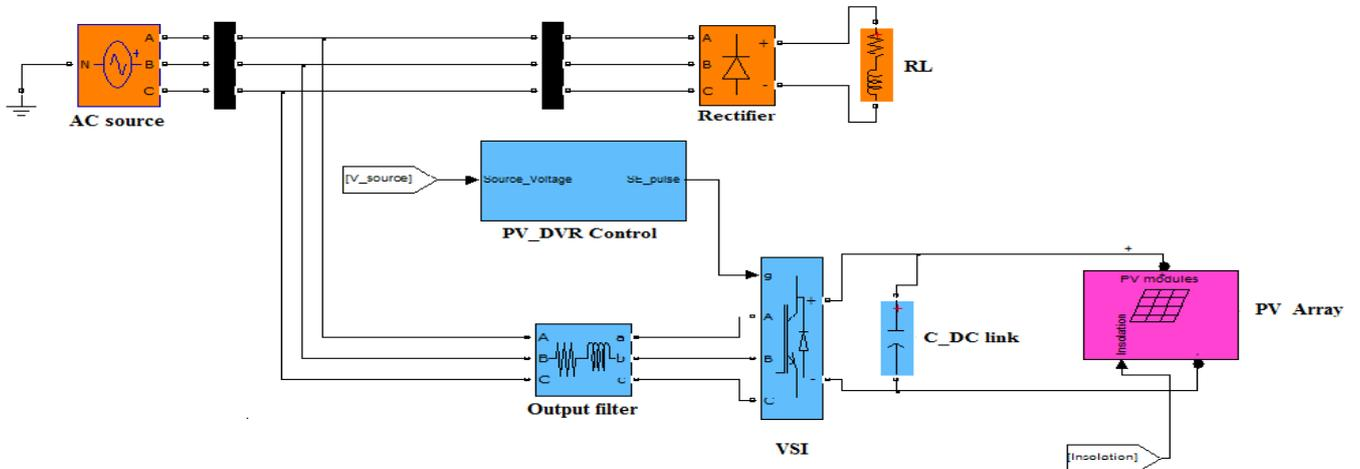
Fig. 5. MATLAB/SIMULINK model for the studied system configuration (PV\_DVR and power system)
