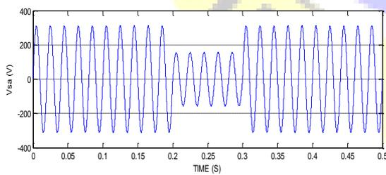
Fig6. Source voltage with 50 % voltage sag in phase A
