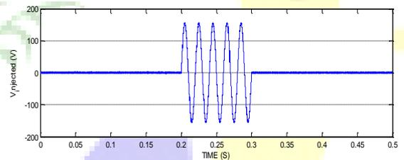
Fig7.DVR injected voltage
