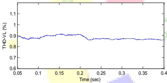
Fig9. Load side total harmonic distortion
