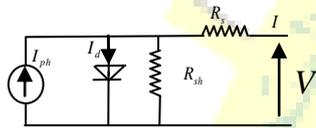
Figure 2: Conventional single diode model.
