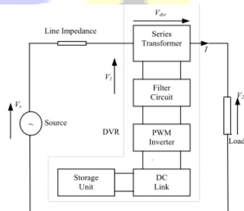
Fig. 1: General structure of power system compensated by dynamic voltage restorer
