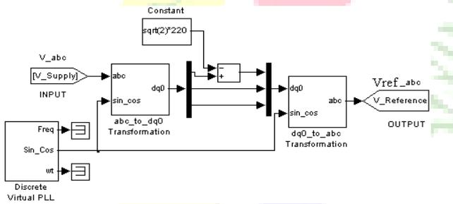
Figure.4. SIMULINK model of SRF method for voltage reference calculation
