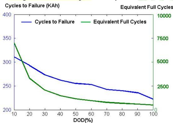
Fig. 3. Battery cycle life vs. depth of discharge
