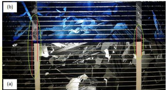
Fig. 5 Photograph of the overlap between the bus-bars.
