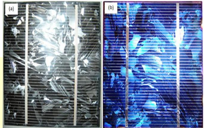
Fig. 2 Photograph of: a) Grid Metallic, b) Grid treated by laser
