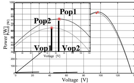
Fig.7 the Maximum Power Point shifting
