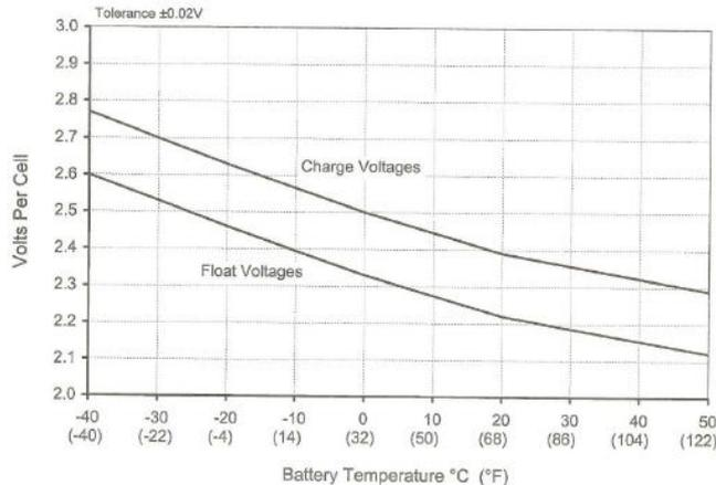
Fig.3. the effect of temperature on the charging process
