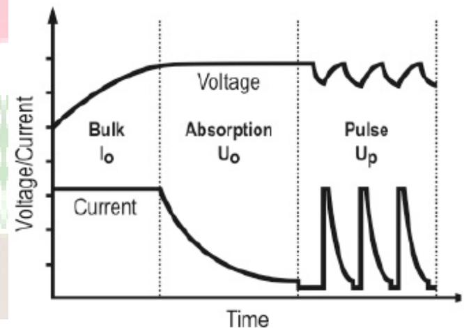
Fig.2. The three-step charge profile
