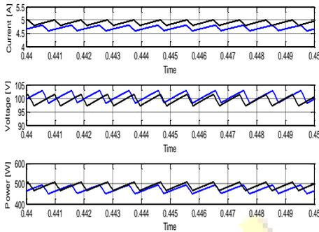
Fig.5 Battery current, voltage and power
