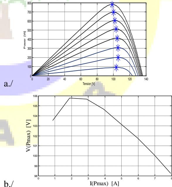
**Fig.1** PV cell's power characteristics (a) and MPP (b)
