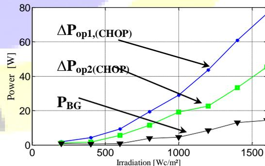
Fig.4 the power chopper consumption
