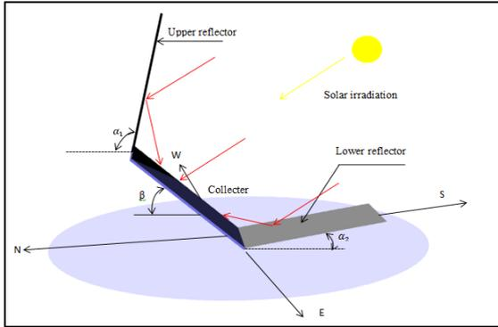
Fig. 1 schematic representation the angles of PVT collector with planer reflector
