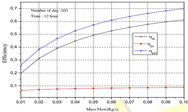
Fig. 9 Effect of mass flow on efficiency of PVT thermal collector with reflectors
