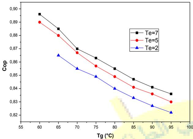
Fig. 2 Variation of the Cop of the system with temperature of generator Tg (Ta and Tc fixed at 30 °C)
