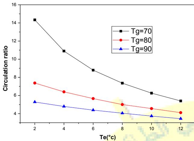
Fig. 6 Effect of generator temperature on the circulation ratio  $\lambda$ .
