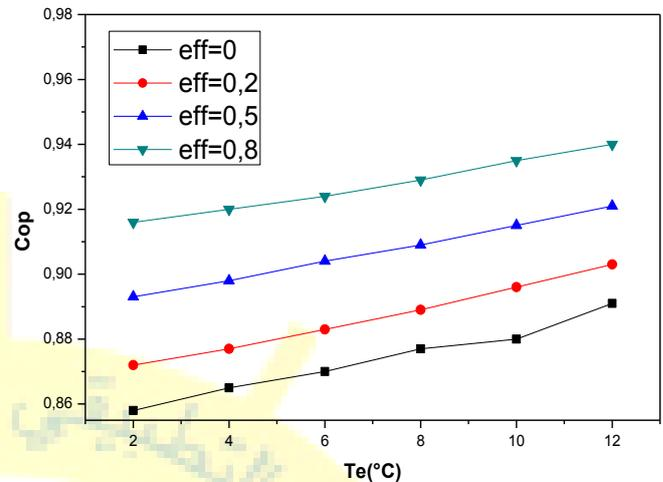
Fig. 4 Effect of efficiency of heat exchanger on coefficient of performance of the system (Tg=70, Tc= 30).
