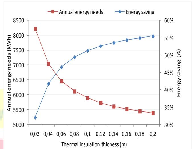
Fig.8. Energy saving at different insulation thickness for ceiling and walls.
