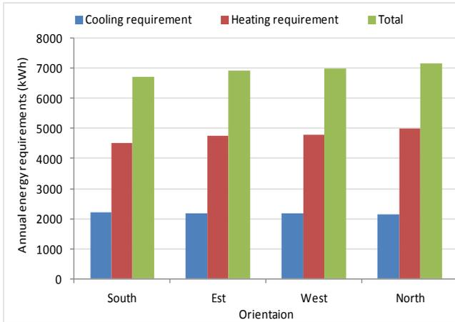
Fig.5. Annual heating and cooling demand at different orientation
