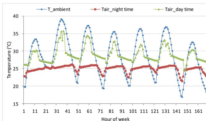
**Fig.9.** Evolution of the temperature in function of time in model house.
