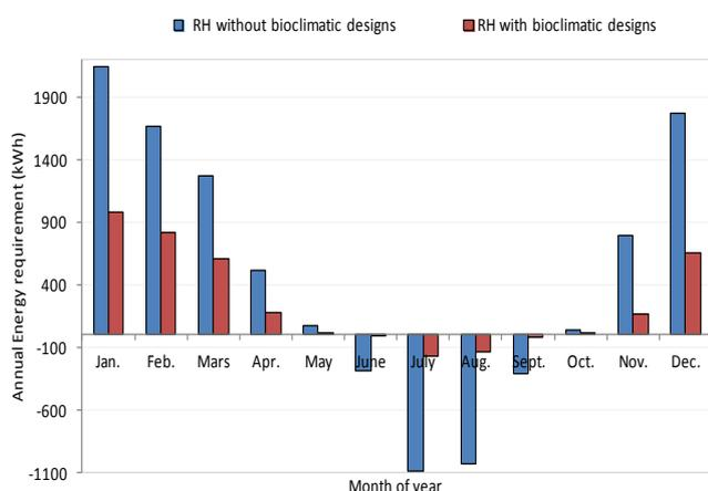
**Fig.10.** Monthly energy requirement comparisons between two houses without and with bioclimatic designs
