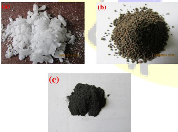
Fig. 1 Sample images of a) PCM and b) expanded clay
