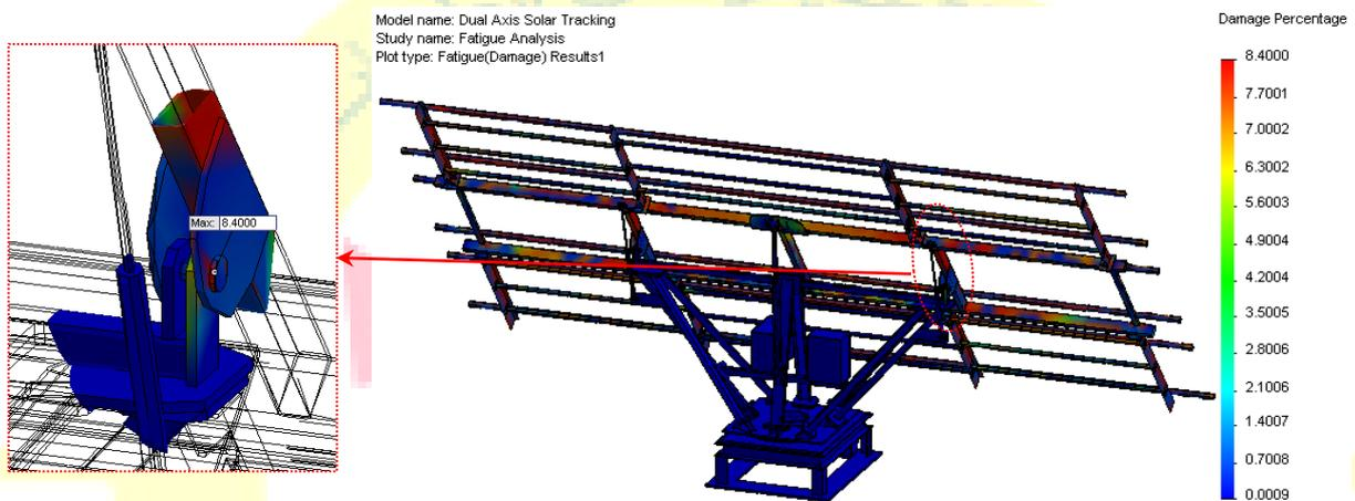
Fig. 5 Damage factor contours of the sun tracking system
