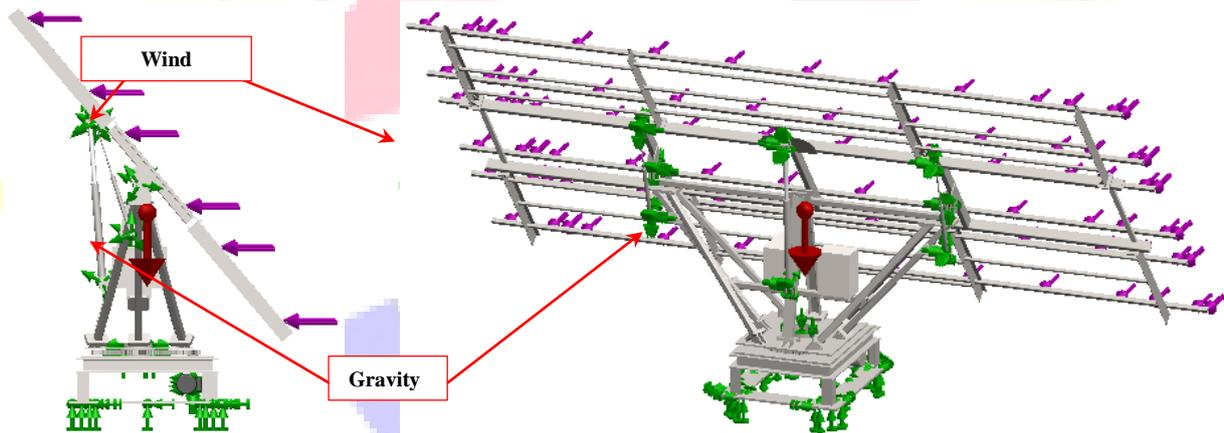
Fig. 1 Loading and boundary condition of the sun tracking system.
