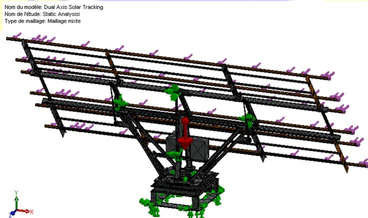
Fig. 2 Finite element mesh model of the sun tracking system.
