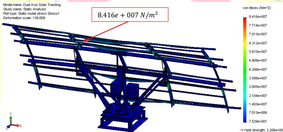
Fig. 3 Von-Mises equivalent stress distribution on the sun tracking system
