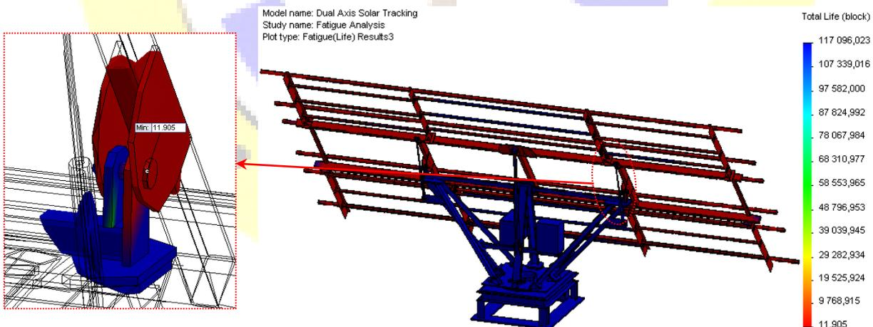
Fig. 6 The fatigue life of the sun tracking system
