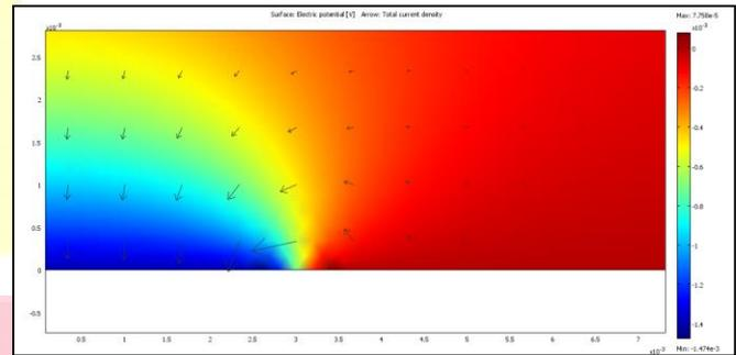
Fig. 4 Surface and arrow plot of electric potential
