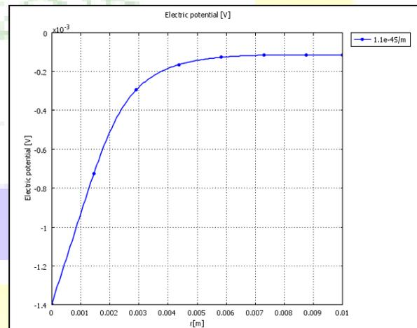
Fig.5. Distibution of electric potential for constant electrical conductivity
