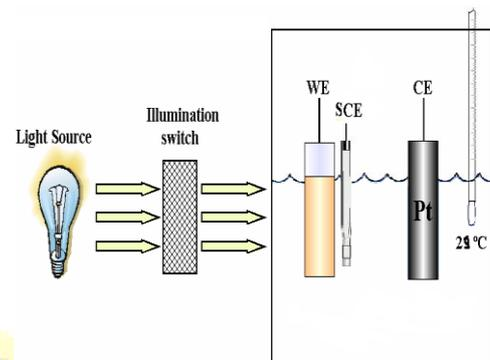
Fig. 2 Arrangement of photocurrent Characterization system
