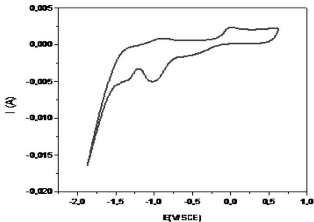
Fig. 3 Cyclic voltammogram of ITO-coated glass for the solution containing 0.01M cupric acetate and 0.1M sodium acetate (pH = 6.2), Scan rate 50 mV s<sup>-1</sup>.
