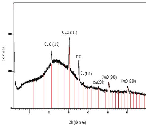
Fig. 4 X-ray diffraction spectra of the films deposited on ITO-coated glass substrate at pH = 6.2.
