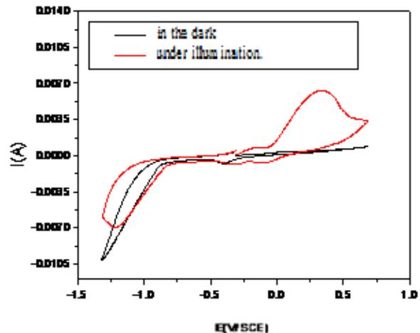
Fig. 5 *Current-Voltage* Characterization of cuprous oxide (Cu<sub>2</sub>O) deposited at -0.50 V vs. SCE for the solution containing 0.1M sodium acetate (CH<sub>3</sub>COONa.3H<sub>2</sub>O) in the dark and under illumination.
