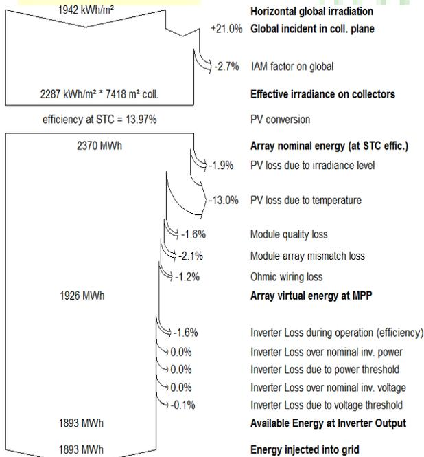
Fig. 12. Diagram of system losses: seasonal tilt
