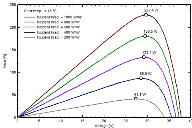
Fig. 3. P-V Characteristics :irradiation effect
