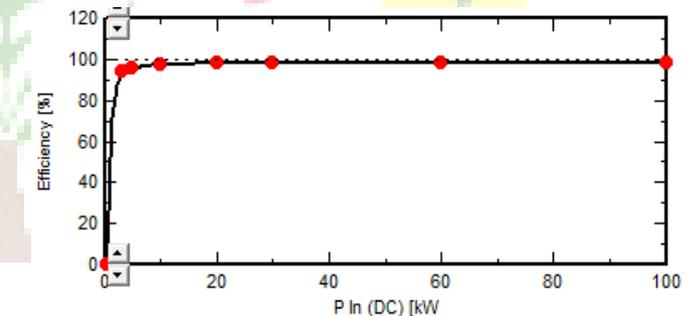
Fig. 5. Efficiency curve of inverter
