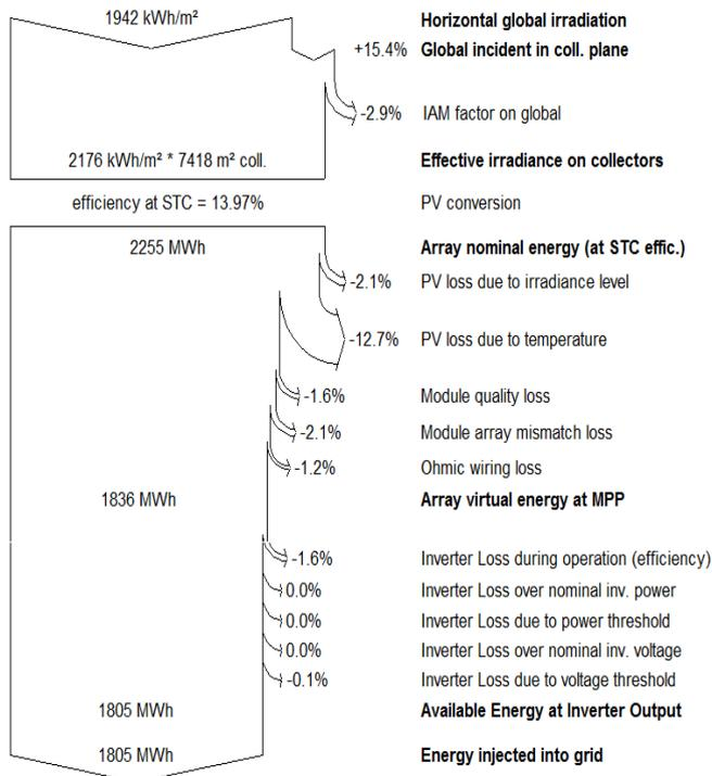
Fig. 11. Diagram of system losses: fixed tilt
