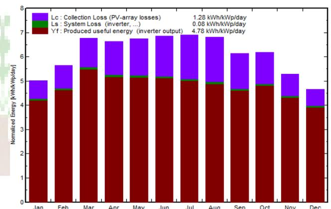
Fig. 9. Loss factors and Normalized production : fixed tilt
