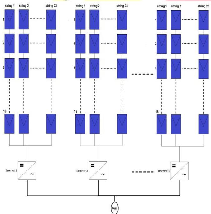
Fig. 8. The proposed model of the plant
