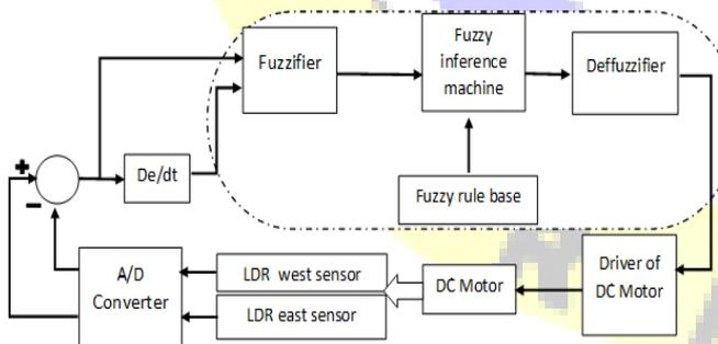
Fig. 4. FLC controller for the sun tracker system.
