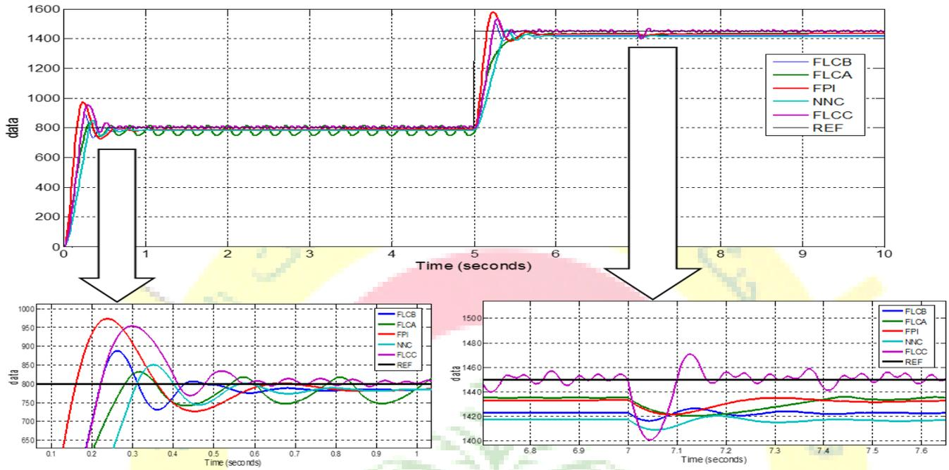
Fig. 19. Comparison between regulators Neural, fuzzy logic and F-PI Controller
