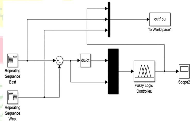
Fig. 8. One Axis Sun Tracker Using FLC<sub>a</sub>
