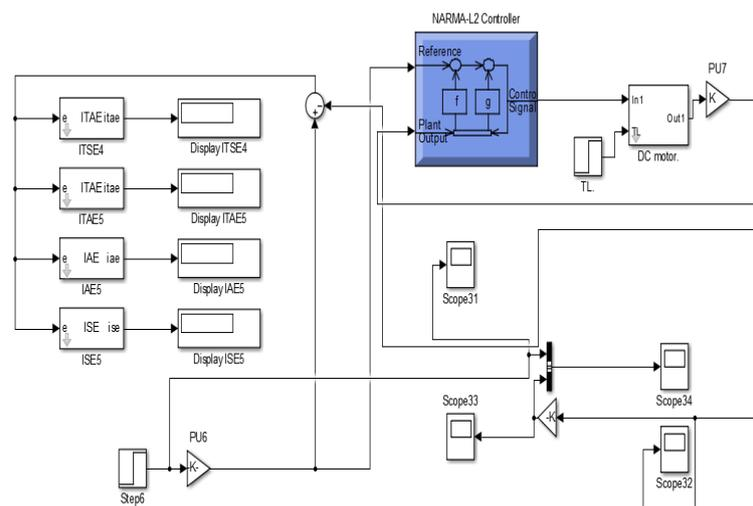
Fig. 16. Closed loop system using Neural Network Controller
