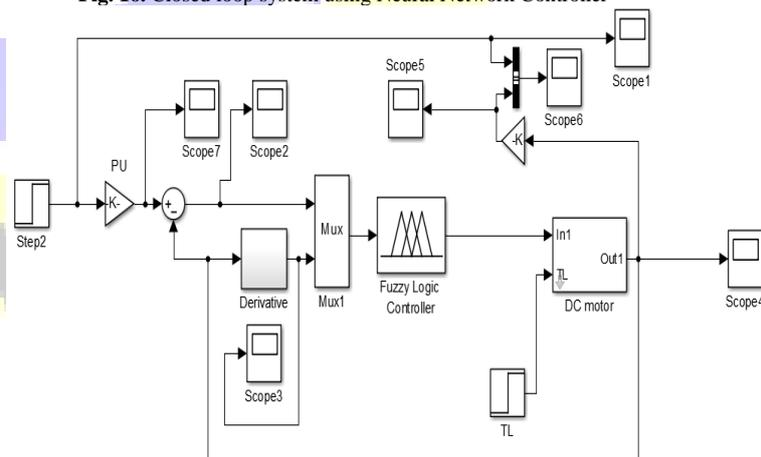
Fig. 17. Closed loop system using Fuzzy logic Controller (FLCA, FLCB, FLCC) [17]
