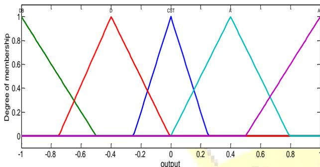
Fig. 10. Fuzzy set of FLC<sub>b</sub> output entering to DC motor driver
