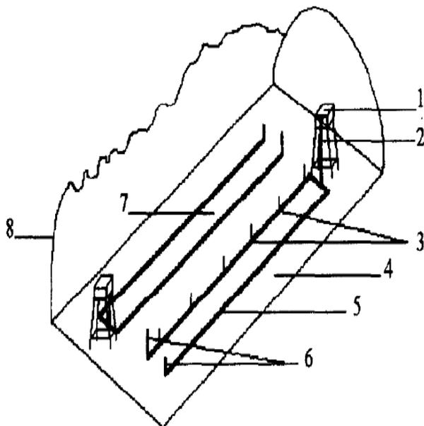
Fig. 2. Storage disposal scheme : 1- Blowers, 2-Pipe inlet, 3- Temperature measurement in pipe, 4- Temperature measurements in soil, 5- pipes filled with gravels, 6- Pipe outlet, 7- Ambient temperature measurements, 8- Greenhouse. . (Bouhdjar et al 1996)
