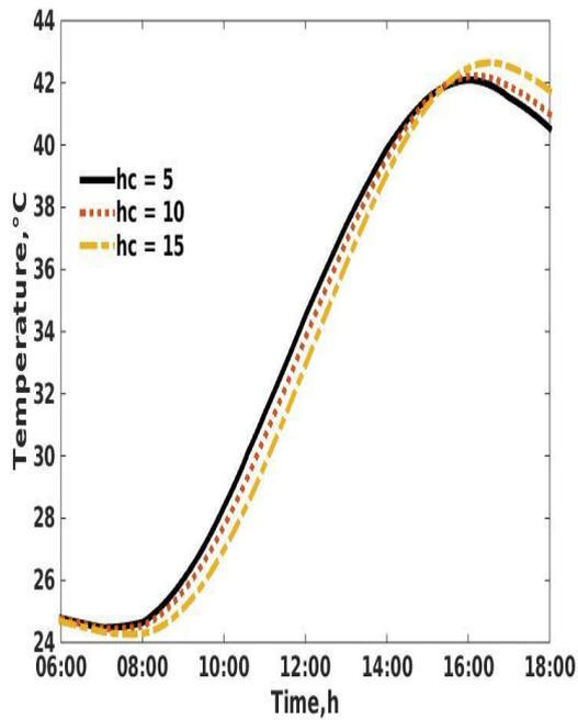
Figure 6. Effect of varying convective heat transfer coefficient.
