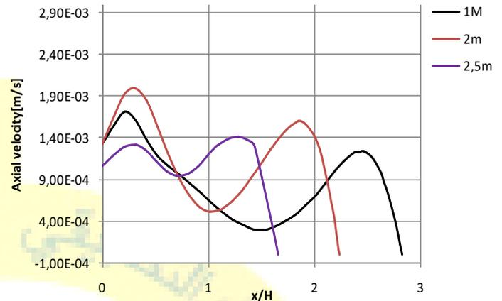
Fig.8. Radial profiles of axial velocity at different sections
