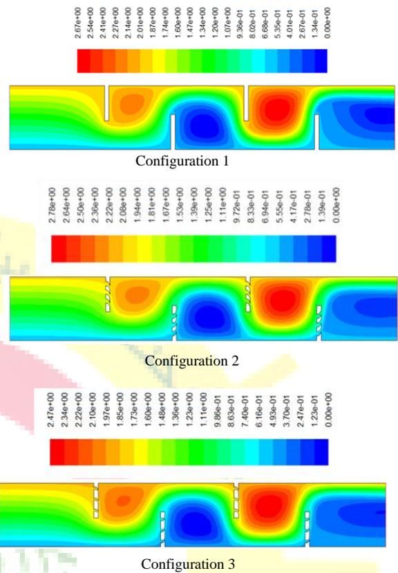
Fig. 3 Contour of streamlines for the three configurations of the solar collector
