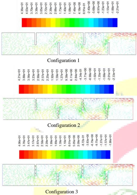
Fig. 4 Contour of pressure coefficient for the three configurations of the solar collector
