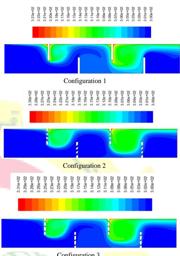
Fig. 5 Contour of temperature for the three configurations of the solar collector
