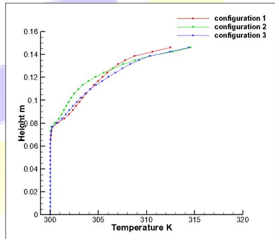
Fig. 6 Profiles of temperature for the three configurations of the solar collector to the position of the section  $x=0.884$  m to the position of the section to the position of the section
