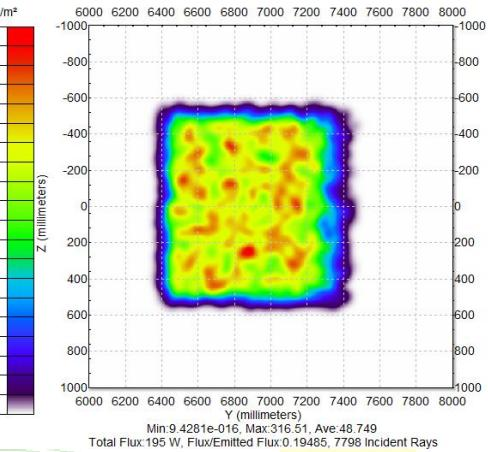
Fig. 3. Reflected irradiance presentation in the absorber from the first heliostat.
