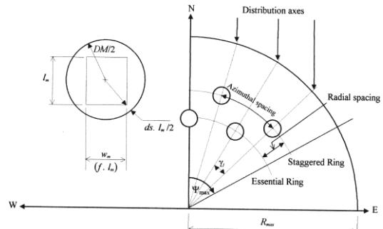
Fig. 1. Fundamental definitions in the heliostat field.
