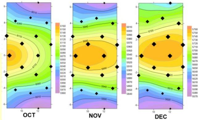
Fig. 5. Yearly irradiation received by each heliostats in the solar field.
