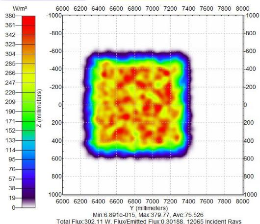
Fig. 4. Reflected irradiance presentation in the absorber from the second heliostat.
