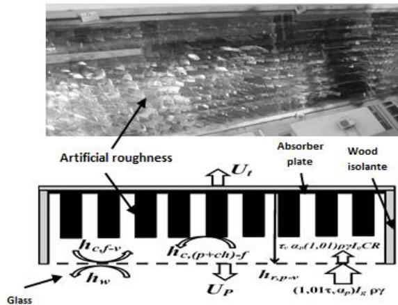
Figure 6: The useful duct absorber with the schema of heat exchange inside it.
