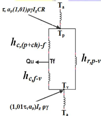
Figure 2 : Electric diagram is equivalent relative to a section of the useful conduit.
