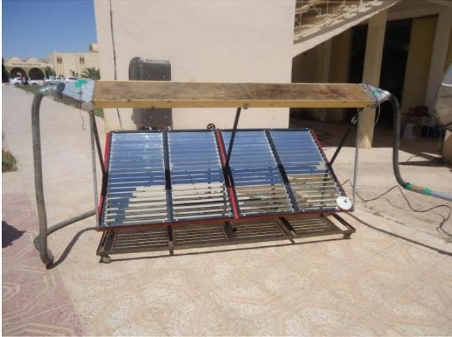
Figure 1: Solar air heater with a Linear Fresnel Reflector (SAHF) with rectangular useful duct absorber.
