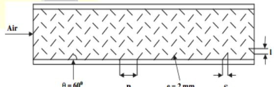
Figure 4 : Roughness in a rectangular channel [6].
