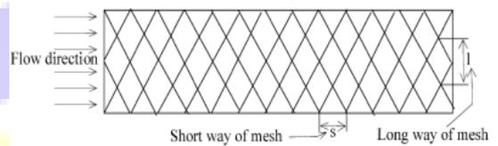
Figure 3 : Grid of artificial roughness [5].
