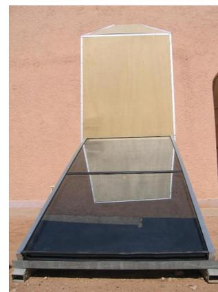
Fig.1 le séchoir solaire indirect
