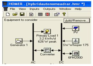
Fig. 1: Proposed hybrid system in HOMER
