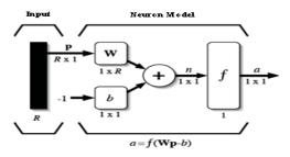
Figure 1. Model of an artificial neuron
