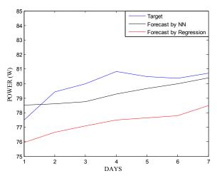
Figure 6. PV Power Forecasting Using Model 2
