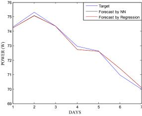
Figure 7. PV Power Forecasting Using Model 3
