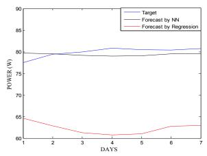
Figure 5. PV Power Forecasting Using Model 1
