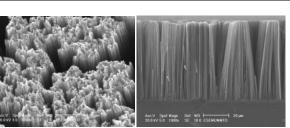
Fig1. Plan (a) and cross section (b)SEM image of p-SiNWs
