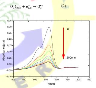
**Fig. 3 UV**/vis absorption spectra of methylene blue before and after UV light irradiation in the presence of the porous SiNWs-Au(80min) substrate as a function of irradiation time
