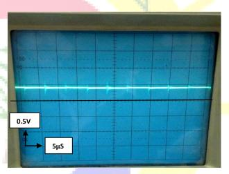
Fig(9-b) Charging current for 17V input voltage
