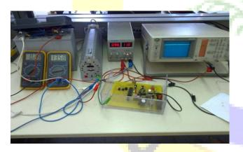
Fig.8 Implemented prototype converter with 12V lead acid battery.
