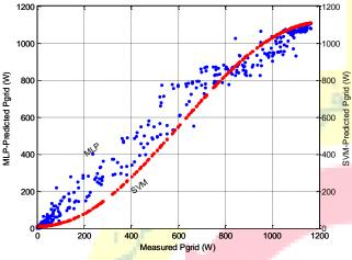
Fig.4 Data of power output and its forecasts by MLP and SVMr
