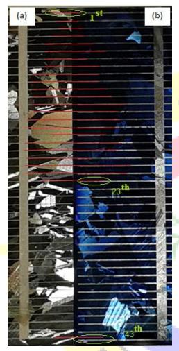
Fig. 4 Photograph of the overlap between the fingers.
