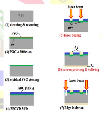
Fig. 1 Process flow for laser tailored selective emitter solar cells. Step 1: The wafer surface is textured with random pyramids. Step 2: POC13 furnace diffusion creates a shallow doped emitter together with a phosphosilicate glass (PSG). Step 3: Hydrofluoric acid removes the PSG layer .Step 4: SiNx anti-reflection coating (ARC) is deposited. Step 5: laser doping. Step 6: Screen printing and firing of the front and back contacts Step 7:edge isolation.
