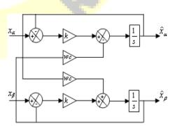
Fig. 2. Self-tuning filter tuned to the pulsation  $w_c$ .
