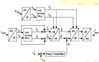
Fig. 3. Block diagram of the new STF-based harmonic isolator.
