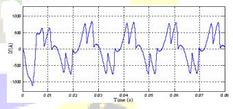
Fig. 9. Active filter current  $I_{f}$ .
