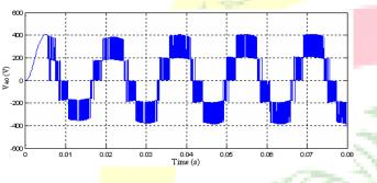
Fig. 12. APF output voltage V<sub>ao</sub>.
