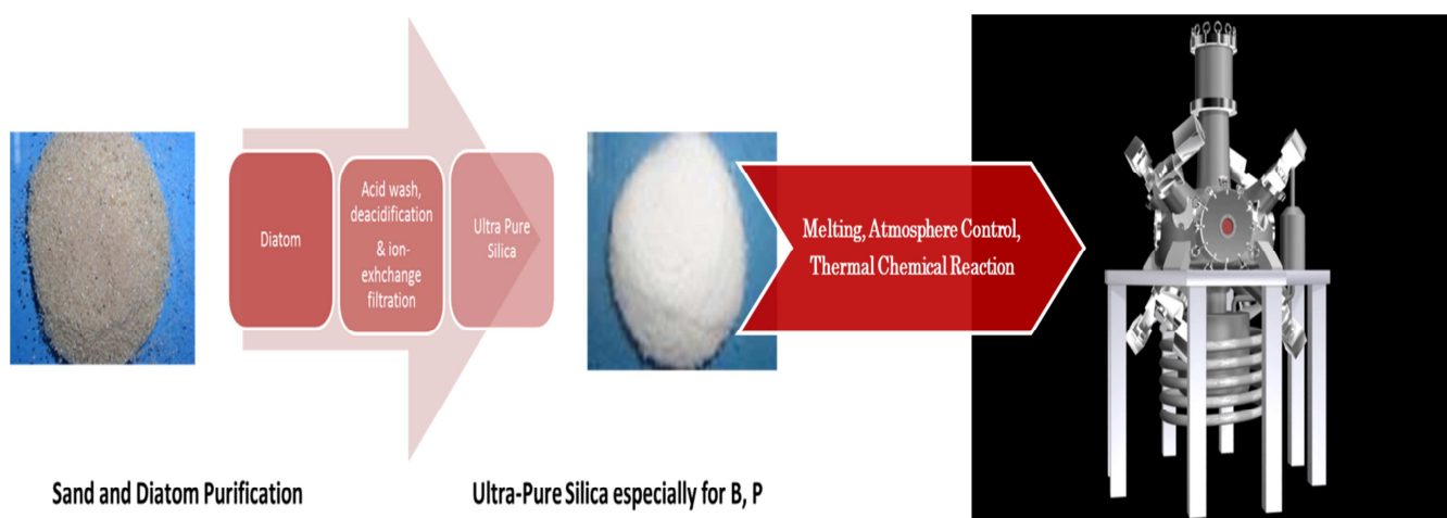
Figure 8: Silica Reduction Concept using microwave heating (One time Reduction by Microwave Heating)
