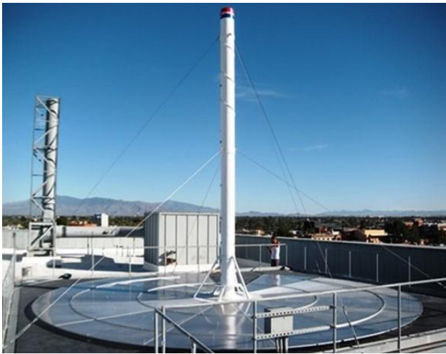
Fig. 14 Prototype de 1:30 scale du prototype de Manzanares, sur le toit de l'Aerospace and Mechanical Engineering Department at University of Arizona, USA [24,25].
