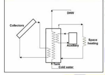
Fig. 1 Top; the pilot house, flat plate solar collectors are installed on the roof of the house facing south (red contour). Bottom; schematic illustration of the solar combisystem serving to domestic hot water supply and space heating
