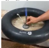
Fig. 8 Flammability test of the biogas
